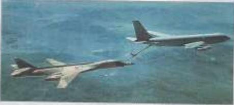
Many human inventions are similar to things already present in nature. The airplane in the picture, for example, is refueling\* through a long, hollow tube similar to a hummingbird's tongue. The Air Force plane at left is receiving fuel directly from a tanker that is flying above it.
